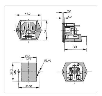
Amperage [A]: 10 Color: Black Connections: 6.3x0.8 Fuse Size [mm]: 5.0x20.0
