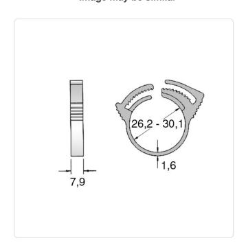
Color: Natural Flammability Class: UL94-V2 PA 6.6 Material: Material Group: Plastic Panel Thickness Range [mm]: 26,2-30,1 1.8
