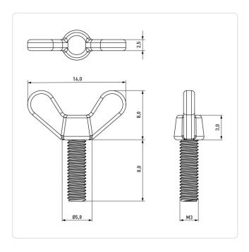
Color: Natural Flammability Class: UL94-V2 Head Diameter [mm]: 16
