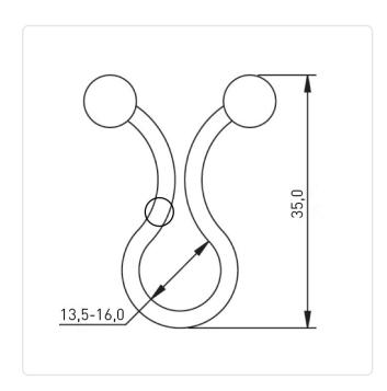
Bundle Diameter [mm]: 10,0-15,0 Color: Natural Flammability Class: UL94-V2 Material: PA 6.6 Material Group: Plastic Weight: 0.77g
