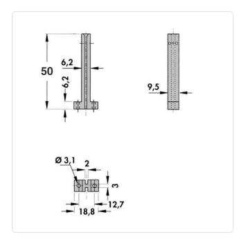
Color: Gray Dist. Mounting Holes [mm]: 12.7 Flammability Class: UL94-V0 Length [mm]: 50
