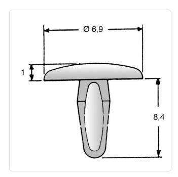
Color: Black Flammability Class: UL94-V2 Head Diameter [mm]: 6.9 Material: PA 6.6 Material Group: **Plastic**
