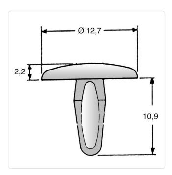
Color: Natural Flammability Class: UL94-V2 Head Diameter [mm]: 12.7 PA 6.6 Material: Material Group: **Plastic** Mounting Hole [mm]: 4.7
