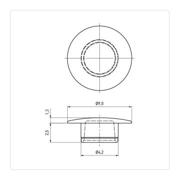
Color: White Head Height [mm]: 1.3 Inner Diameter [mm]: 4.2
