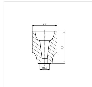
Inner Diameter [mm]: 4.6 Length [mm]: 8 Material: Ceramic C221 Material Group: Ceramic C221 Model: With Lug Outer Diameter [mm]: 9 Weight: 0.59g Conformities: Reach RoHS **SVHC**
