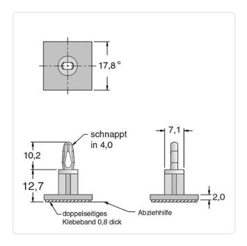
Color: Natural Flammability Class: UL94-V2 Length [mm]: 12.7 Material: PA 6.6 Material Group: **Plastic** PCB Hole Ø [mm]: PCB Thickness [mm]: 1,6 Weight: 1.09g
