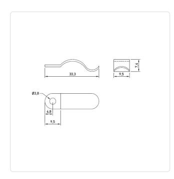
Bundle Diameter [mm]: 5,9 Color: Black Flammability Class: UL94-V2 Length [mm]: 33.3 Material: PA 6.6 **Plastic** Material Group: Mounting Hole [mm]: 3.8 Width [mm]: 9.5 Weight: 0.41g
