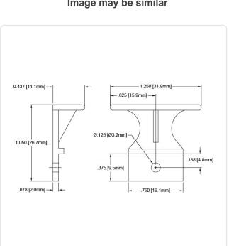
White Color: Flammability Class: UL94-V2 31.8 Length [mm]: Material: PA 6.6 **Plastic** Material Group: 11.1 Width [mm]: Weight: 1.84g
