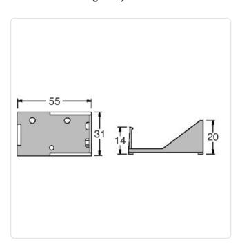
Battery Type: C-Baby Flammability Class: UL94-HB
