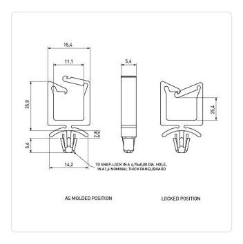
Bundle Diameter [mm]: 10,0-25,0 Color: Natural Height [mm]: 35.1 PA 6.6 Material: Material Group: **Plastic** Mounting Hole [mm]: 4.8 Panel Thickness [mm]: 1,6 mm 15.4 Width [mm]: Weight: 1.32g
