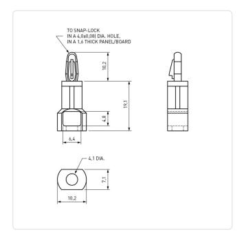
Color: Natural UL94-V2 Flammability Class: 19.1 Length [mm]: PA 6.6 Material: Material Group: **Plastic** PCB Hole Ø [mm]: PCB Thickness [mm]: 1,6 Panel Hole Ø [mm]: 4.1 Weight: 0.63g
