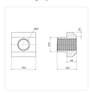
DIN/ISO: **DIN508** Plain Finish: Head Height [mm]: 8 Height [mm]: 16
