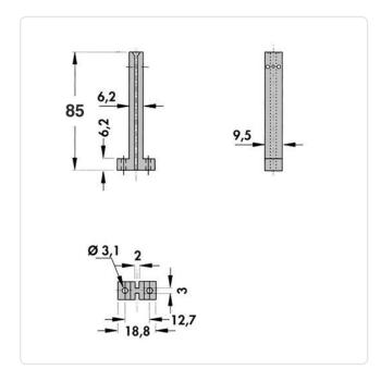
Color: Gray Dist. Mounting Holes [mm]: 12.7 Flammability Class: UL94-V0 Length [mm]: 85
