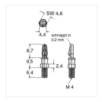
Color: Natural Flammability Class: UL94-V2 Length [mm]: 9.5 Material: PA 6.6 Material Group: **Plastic** PCB Hole Ø [mm]: 3.2 PCB Thickness [mm]: 1,6 Thread Size: M4 Weight: 0.27g
