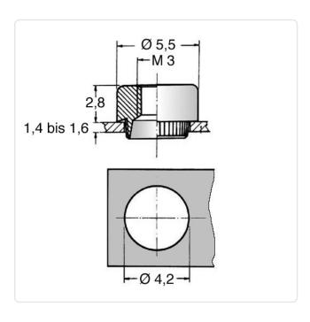
Finish: Plain Height [mm]: 2.8 Material: Steel Material Group: Steel Outer Diameter [mm]: 5.5 Panel Hole Ø [mm]: 4.2 Panel Thickness [mm]: 1,4 - 1,6 Thread Size: М3 Weight: 0.43g
