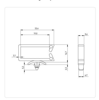
Bundle Diameter [mm]: 10,0-25,0 Color: Natural Height [mm]: 16.7 Material: PA 6.6 Material Group: **Plastic** Mounting Hole [mm]: 4.8 Width [mm]: 25.5
