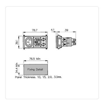
Amperage [A]: 10 Color: Black Connections: 6.3x0.8 Fuse Size [mm]: 5.0x20.0 Weight: 56.8g
