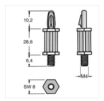
Color: Natural Flammability Class: UL94-V2 28.6 Length [mm]: Material: PA 6.6 Material Group: **Plastic** PCB Hole Ø [mm]: PCB Thickness [mm]: 1,6 Thread Size: M4 Weight: 1.1g
