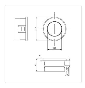
Color: Black Inner Diameter [mm]: 16 Material: PA 6.6 Material Group: Plastic Max. Panel Thickness [mm]: 1.6 Mounting Hole [mm]: 19 Outer Diameter [mm]: 21 Weight: 0.57g
