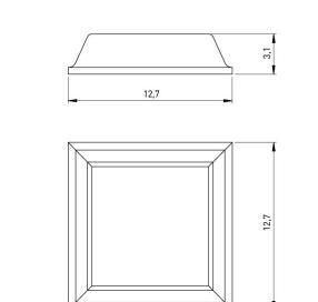
Bumper Design:Square, TColor:GrayDiameter [mm]:12.7Flammability Class:UL94-HBHeight [mm]:3.1Material:PUR - PolMaterial Group:PlasticWeight:0.55gConformities:Reach
