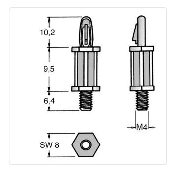
Color: Natural Flammability Class: UL94-V2 9.5 Length [mm]: Material: PA 6.6 Material Group: **Plastic** PCB Hole Ø [mm]: PCB Thickness [mm]: 1,6 Thread Size: M4 Weight: 0.5g
