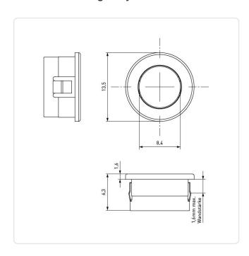
Color: Black Inner Diameter [mm]: 8.8 Material: PA 6.6 Material Group: Plastic Max. Panel Thickness [mm]: 1.6 Mounting Hole [mm]: 11.9 Outer Diameter [mm]: 13.5 Weight: 0.35g
