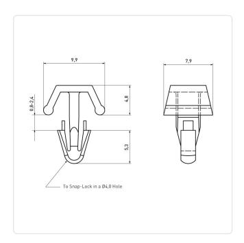
Color: Natural Flammability Class: UL94-V2 Head Diameter [mm]: 9.9 Material: PA 6.6 Material Group: Plastic
