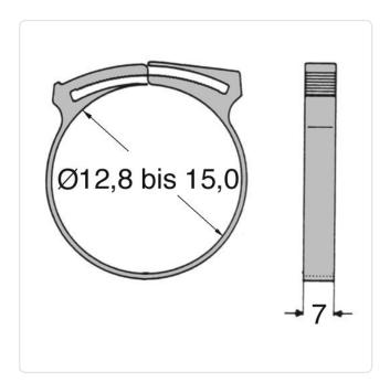
Color: Black Flammability Class: UL94-V2 PA 6.6 Material: Material Group: Plastic Panel Thickness Range [mm]: 12,8-15,0
