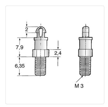
Color: Natural Flammability Class: UL94-V2 Length [mm]: 7.9 Material: PA 6.6 Material Group: **Plastic** PCB Hole Ø [mm]: 2.5 PCB Thickness [mm]: 1,6 Thread Size: М3 Weight: 0.19g
