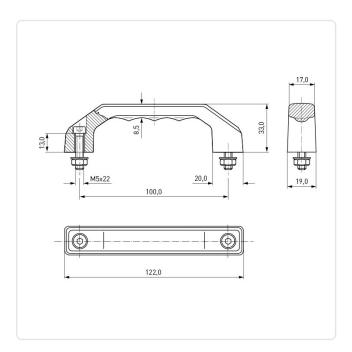
Color: Black Dist. Mounting Holes [mm]: 100 Height [mm]: 33 Material: PA 6.0 Material Group: Plastic
