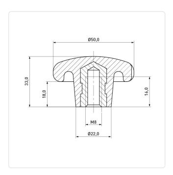
Color: Black Diameter [mm]: 50 Height [mm]: Material: Plastic Material Group: Plastic Thread Size: M8
