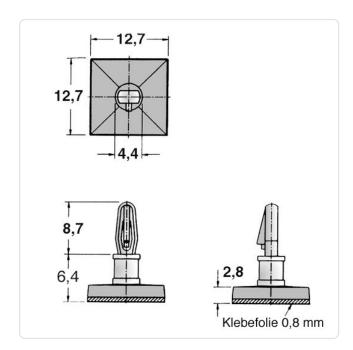
Color: Natural Flammability Class: UL94-V2 Length [mm]: 6.4 Material: PA 6.6 Material Group: **Plastic** PCB Hole Ø [mm]: 3.2 PCB Thickness [mm]: 1,6
