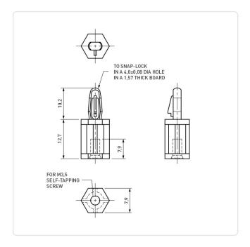
Color: Natural Flammability Class: UL94-V2 12.7 Length [mm]: PA 6.6 Material: Material Group: **Plastic** PCB Hole Ø [mm]: PCB Thickness [mm]: 1,6 Thread Size: M3.5 Weight: 0.55g
