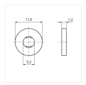
Color: Red For Thread Size: M5 Height [mm]: 1.3 Inner Diameter [mm]: 5.3
