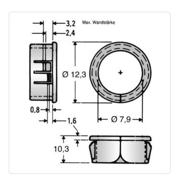
Color: Black Inner Diameter [mm]: 7.9 Material: PA 6.6 Plastic Material Group: Max. Panel Thickness [mm]: 3.2 Mounting Hole [mm]: 11.1 Outer Diameter [mm]: 12.3 Weight: 0.36g
