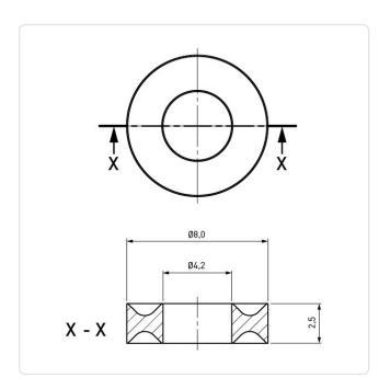
For Thread Size: M4 2.5 Height [mm]: Inner Diameter [mm]: 4.2 Material: PA 6.0 Material Group: **Plastic** Outer Diameter [mm]: 8
