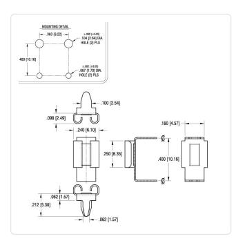
Amperage [A]: 30 Fuse Size [mm]: 5.2x0.64 Material: **Brass** Material Group: **Brass**
