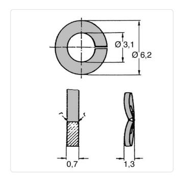
DIN/ISO: DIN128A Finish: Plain For Thread Size: M3 0.7 Height [mm]: Inner Diameter [mm]: 3.1
