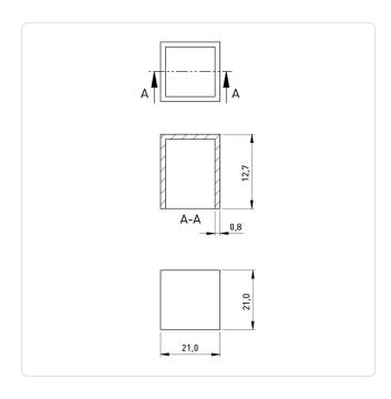
Color: Black Flammability Class: UL94-V2 Height [mm]: 12.7 Length [mm]: 21 PA 6.6 Material: Material Group: Plastic
