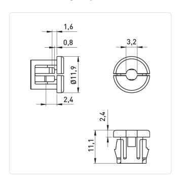
Color: Black Inner Diameter [mm]: 3.2 Material: PA 6.6 Material Group: Plastic Max. Panel Thickness [mm]: 3.2 Mounting Hole [mm]: 10 Outer Diameter [mm]: 11.9 Weight: 0.54g
