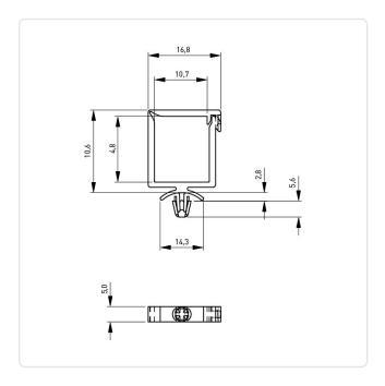
Bundle Diameter [mm]: 10,0-18,0 Color: Natural Height [mm]: 10.6 Material: PA 6.6 Material Group: **Plastic** Model: Folding Mounting Hole [mm]: 4.8
