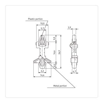
Color: Black Flammability Class: UL94-V0 14.4 Length [mm]: PA 6.6 Material: Material Group: **Plastic** PCB Hole Ø [mm]: PCB Thickness [mm]: 1,6 Panel Hole Ø [mm]: 4.8
