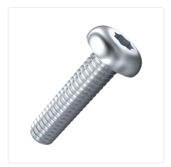
Actuator Size: Torx T10 DIN/ISO: ISO7380-1 Drive Type: **TORX** Plain Finish: Head Diameter [mm]: 5.7 Head Height [mm]: 1.65
