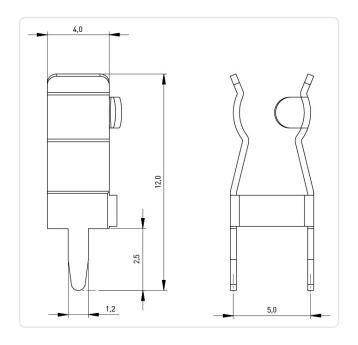
Fuse Size [mm]: 5.0x20.0 Material: **Brass** Material Group: Brass Clip Holder Model:
