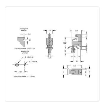
Color: Natural Flammability Class: UL94-V2 12.2 Length [mm]: PA 6.6 Material: Material Group: **Plastic** 1,6-2,3 PCB Thickness [mm]: Panel Hole Ø [mm]: 4.8 Panel Thickness [mm]: 1,0-2,3 Weight: 0.82g
