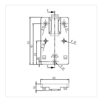
Color: Black Flammability Class: UL94-V0 Height [mm]: 10.5 75.2 Length [mm]: PA 6.0 Material: Material Group: **Plastic** Width [mm]: 45
