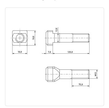
DIN/ISO: **DIN787** Finish: Plain Head Height [mm]:
