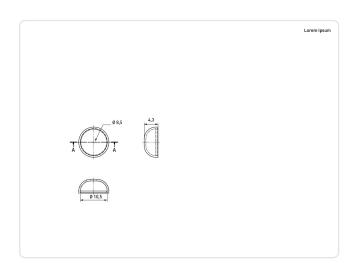
Color: Black Head Height [mm]: 4.3 Inner Diameter [mm]: 8.5 PA 6.0 Material: Material Group: **Plastic**
