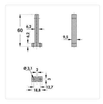
Color: Gray Dist. Mounting Holes [mm]: 12.7 Flammability Class: UL94-V0 Length [mm]: 60
