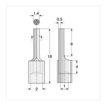
Color: Yellow DIN/ISO: DIN46231-A Finish: Tin-Plated Insulation: Polyamide
